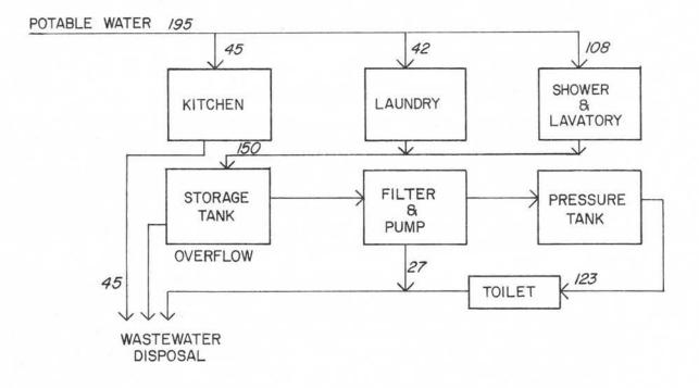
FIGURE 6.1.2-A. TYPICAL GREY WATER SYSTEM - Numbers indicate daily water consumption (gallons) for an average family of three.
